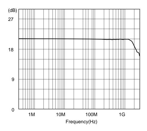
(2) Dependence of Gain and High Frequency Cutoff on Power Supply Variations  $\rm T_a$  =25 °C, V $_{DD}$  =-5 V, V $_{SS}$  =GND, Pin =-40 dBm, RL =50  $\Omega$ ,300 kHz-3 GHz
